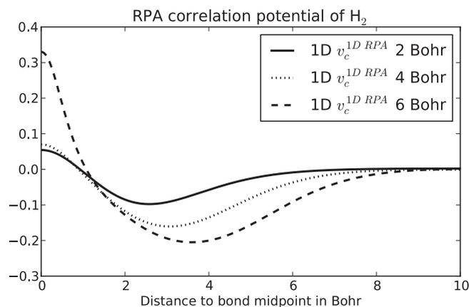
FIG. 4. The correlation potential along the bond axis with the bond midpoint at zero. The system is 1D  $H_2$  with a soft Coulomb potential.
