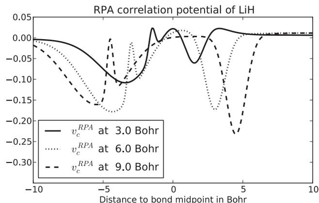
FIG. 7. The correlation potential of LiH along the bond axis. The bond midpoint is at zero. The Li atom is located at  $-1.5$ ,  $-2.5$ , and  $-4$  bohrs, respectively. The H atom is located at  $1.5$ ,  $2.5$ , and  $4$  bohrs, respectively.
