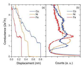
FIG. 1. (Color online) (a) Typical traces of conductance for breaking contacts of Co, Fe, and Ni. (b) Histograms of conductance are constructed from thousands of these breaking traces of contacts fabricated by STM at 4.2 K for Ni, Fe, or Co. The histograms for the three materials show a clear first peak at values above  $2e^2/h$ .
