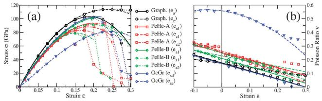
Fig. 2 (a) Stress-strain curves and (b) Poisson's ratios as a function of strain, for graphene, PeHe-A, PeHe-B, and OcGr for different strain directions. The straight, dashed and dot-dashed lines in the stress-strain graph are the fitting lines according to eqn (1) and (2) for (a) and (b), respectively. The dotted lines in (a) connect the stress-strain points for strain values  $\varepsilon \gtrsim \varepsilon_u$ .
