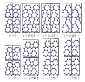
Fig. 5 Snapshots of PeHe-A for specific strains along  $e_{\rm z1}$  (top) and  $e_{\rm a1}$  (bottom). The arrows show the strain direction.
