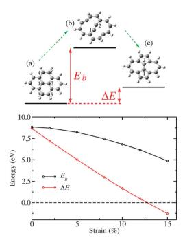
Fig. 11 The transition diagram of pyrene molecule (top), as well as the transition state energy  $E_{\rm b}$  and the energy difference  $\Delta E$  of (c) from (a) as a function of uniaxial strain (bottom).
