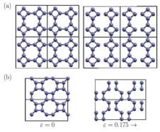
**Fig. 4** Snapshots of OcGr for specific strain values along (a)  $e_{sd}$  and (b)  $e_{se}$  directions. Bonds start breaking in both cases at  $\varepsilon = 0.175$ . The arrows next to the strain values indicate the strain direction.
