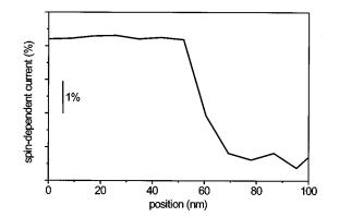
FIG. 4. Line scan across a domain wall between two domains of opposite contrast on Co(0001). The displayed data is raw data of a single scan and was recorded in  $\approx 100$  ms.
