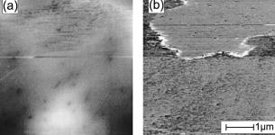
FIG. 1. STM images of the topography (a) the magnetic domain structure of the same area (b) of polycrystalline Ni. Sample bias: 0.13 V; tunneling current: 1 nA; (a) height variations 3 nm; (b) spin contrast: 2.2%.
