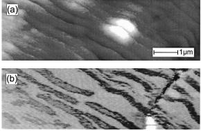
FIG. 3. STM images of the topography (a) the magnetic domain structure of the same area (b) of Co(0001). Sample bias: 0.2 V; tunneling current: 0.5 nA; (a) height variations 4 nm; (b) spin contrast: 3.6%.
