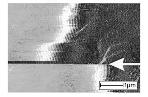
FIG. 2. STM image of a domain wall at the surface of Co(0001). When applying an external magnetic field pulse of 50 Oe (indicated by the arrow), the domain wall is moved to the left during scanning. Sample bias: 0.2 V.
