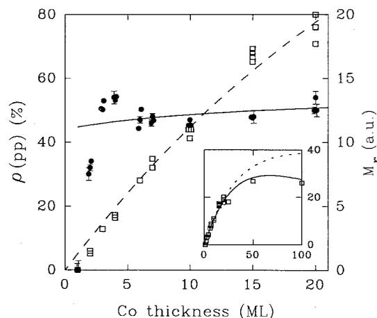
Fig. 1. Co film thickness dependence of the relative nonlinear magnetic effect  $\rho$  (pp) and the MOKE amplitude  $M_r$  in Co/Cu(001); dots/solid line - experimental  $\rho$  (pp) data and theoretical fit; open symbols/dashed line - MOKE data and fit. The inset shows the MOKE data and fits for thicker Co films; dashed line: Lambert Beer's law, solid line: multiple reflection model.
