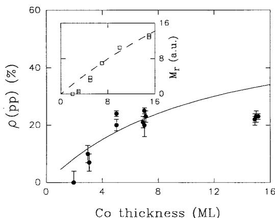
Fig. 3. Calculated and experimental Co film thickness dependence of  $\rho$  (pp) in Cu/Co/Cu(001); dots – experimental data; solid line – calculation based on fitting parameters of Fig. 1. The inset shows the experimental and calculated MOKE amplitude.
