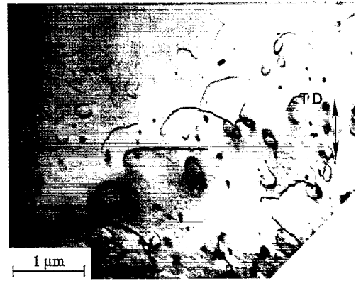
Fig. 12. Dislocation structure during in situ straining in [100] direction (TD) at 1150°C. Foil surfaces (001) .
