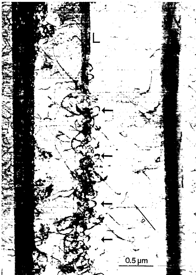
Fig. 10. Dislocation structure in nearly lamellar Ti-Al after unloading an in situ specimen deformed at 900 K. Multiplication processes (arrow) at interface dislocations at the site of a former lamella (L), which receded during thermal treatment.
