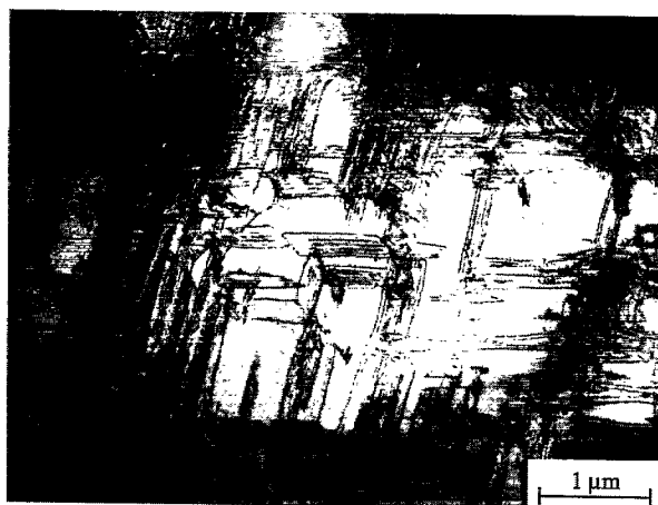
Fig. 14. Dislocations and planar faults in PSZ containing 6.8 mol% Y_2O_3 being annealed at 1600°C for 50 h and deformed at 1400°C. After [32].
