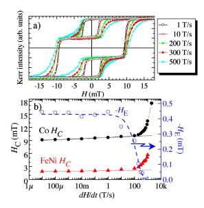
FIG. 2. (Color online) (a) Hysteresis loops of the Co(5 nm)/Cu(10 nm)/FeNi(5 nm) spin valve measured along the easy axis for several field sweep rates dH/dt. (b) dH/dt dependence of the coercivities  $H_C$  of the FeNi and Co films and of the interlayer magnetic coupling  $H_E$  obtained from the shift of the minor hysteresis loop of the FeNi layer. The lines are guides to the eye.
