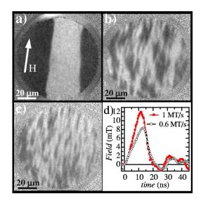
FIG. 3. (Color online) X-PEEM images showing the domain structure of the permalloy layer of the spin valve sample after application of magnetic pulses: (a) pulse 1 ms long and 2 mT high; (b) and (c) pulses 20 ns long with sweep rate values and amplitudes shown in panel (d). The pulsed field direction is indicated in (a) and is parallel to the easy magnetization axis.
