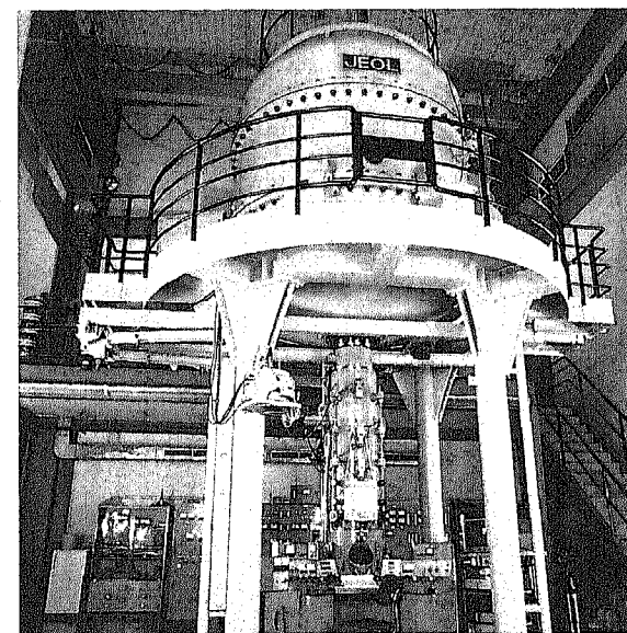
Fig.1. The JEOL 1000 kV high-voltage transmission electron microscope installed in Halle (Saale), Germany.
