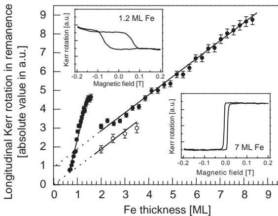
Fig. 3. Thickness dependence of remanent Kerr rotation measured along the [1 0 0] direction at 60 K for Fe films grown on Pd/Cu(001) (full dots) and Cu(001) (open circles). The data for Fe grown on Cu(001) is shown only in the thickness range the films are magnetized in plane and do not experience any structural transformation (2–4 ML). The slope of both linear dependencies is the same. The positive offset in the case of Fe/Pd/Cu(001) system corresponds to about 1 ML of Fe.
