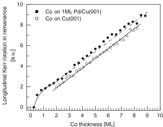
Fig. 2. Thickness dependence of remanent MOKE rotation measured along the [100] direction at 70 K for Co films grown on Pd/Cu(001) (full dots) and Cu(001) (open circles). The slope of both linear dependencies is almost the same. The positive offset in the case of Co/Pd/Cu(001) system corresponds to the signal from about 0.6 ML of Co.
