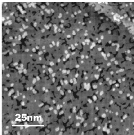
Fig. 1. STM image of 1 ML Co on 1 ML Pd/Cu(001). The Co layer was grown by thermal deposition at RT. Only a few small islands of 1 ML height are seen confirming almost perfect layer-by-layer growth.
