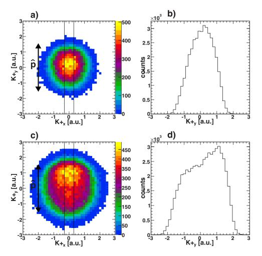
FIG. 6. (Color online) Centerof-mass momentum distribution parallel to the surface for  $\hbar\omega$ =40 and 60 eV. The sum energy is set to 30 and 50 eV, respectively. [(a) and (c)] Full 2D distributions and [(b) and (d)] projection of the area between the vertical lines to the y axis.
