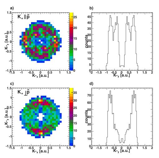
FIG. 7. (Color online) Distribution of relative momenta for different orientations of the sum momentum in respect to the polarization vector.  $\hbar\omega$  is 40 eV and sum energies  $E_1+E_2=\hbar\omega$  $-2W_{\phi}\pm 3$  eV, equal energy sharing. (a) Sum momentum parallel to polarization and (c) sum momentum perpendicular to polarization. (b) and (d) are projections of the area  $K_{-x}\pm 0.3$  a.u. to the Y axis.
