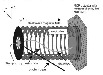
FIG. 1. Sketch of the experimental setup. The spectrometer axis lies along the *z* axis, and the sample in the *XY* plane. The light incidence angle is  $45^{\circ}$  to the surface normal with the polarization in the *YZ* plane.
