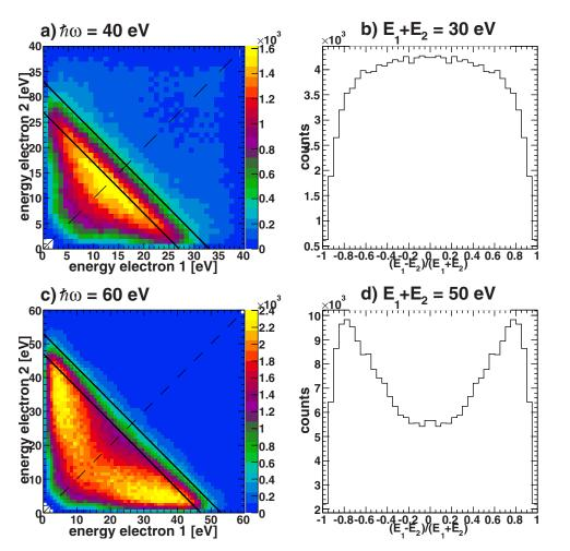
FIG. 2. (Color online) [(a) and (c)] Electron-electron energy spectrum for  $\hbar \omega = 40$  and 60 eV; the spectra have been mirrored at the diagonal broken line. [(b) and (d)] Electron energy sharing [ $(E_1 - E_2)/(E_1 + E_2)$ ] for sum energies in the area between the two solid lines.
